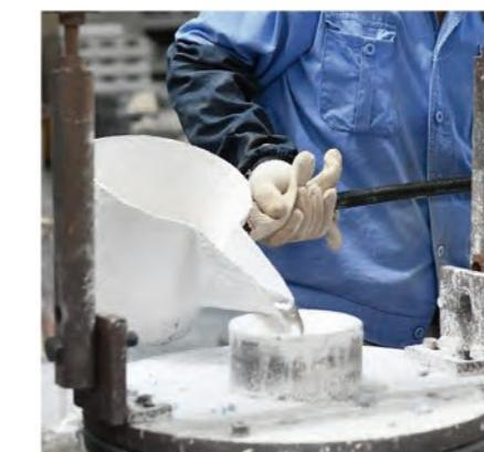
We manufacture gravity casting of aluminum alloy. All process are managed in an integrated production systems within our factory, therefore we achieve that a high quality, low cost and the shortest delivery time.
