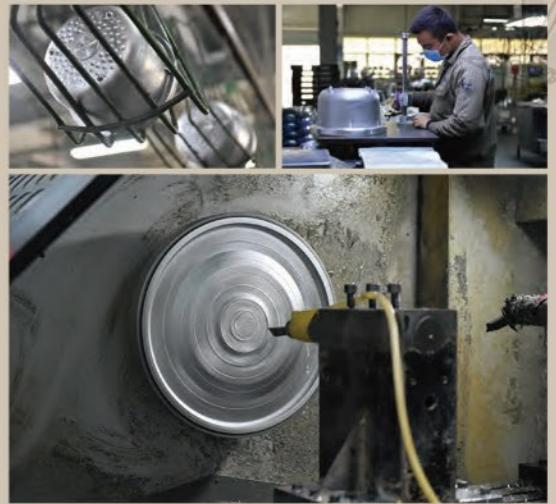
The casting products manufactured by gravity mould casting, the crystal structure is miniaturized on the surface, and the porous tissue is formed inside. Not only controlling of temperature, moisture and the speed, also by the craftsman's own strong desire, with accumulated excellent experiences and high technology skills, excellent castings are created.
