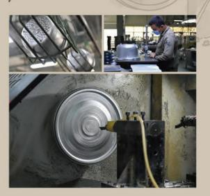
In order to realize the precise size requirements, each piece is carefully carved by a computer-controlled NC cutting machine.It is possible to crave castings wall thickness into variable shapes. The [thick bottom thin wall structure] is most suitable for the cooking utensils. It requires dense calculation and technology in order to prevent bottom sagging deformation due to heat and to exert the water sealing effect of dry cooking.
